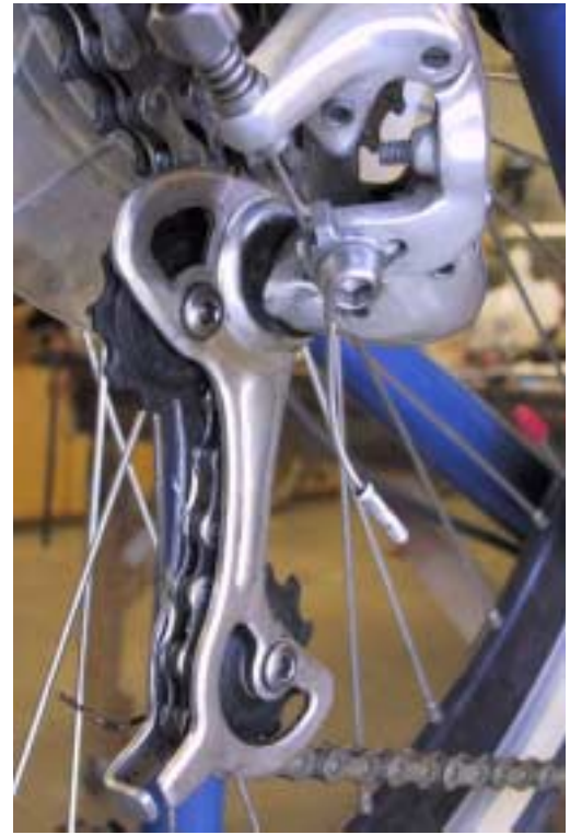
Campy long cage derailleur. This is the 9 speed racing T derailleur used with an 8 speed Shimano cassette. The levers are 9 speed Campy Chorus
