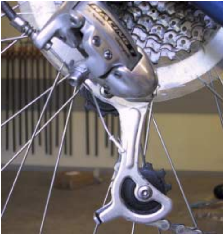
Campy long cage derailleur. This is the 9 speed racing T derailleur used with an 8 speed Shimano cassette. The levers are 9 speed Campy Chorus
