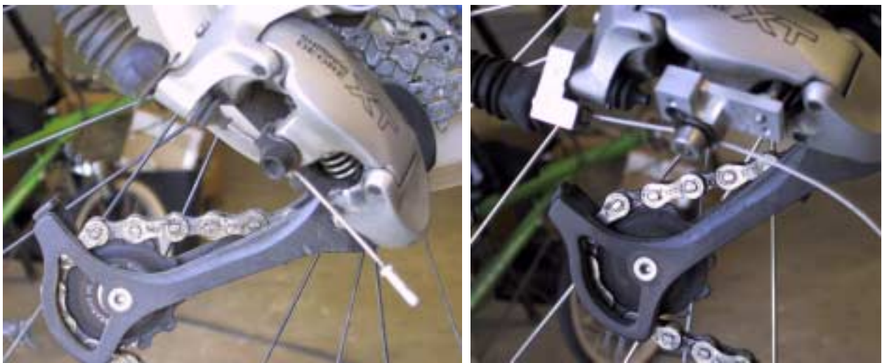
On the left, a standard XT derailleur. On the right, the XT Derailleur with the VeloParts Inc. adapter installed
